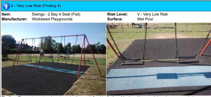
**Finding:** The seats are too close to each other as defined in **Action:** Monitor - No remedial work recommended BS EN 1176 Part 2; this is a low risk failure and no remedial action is required
