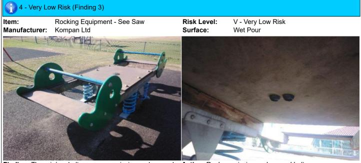
**Finding:** There is/are bolt cap covers missing or damaged **Action:** Replace missing or damaged bolt cap covers on the item
