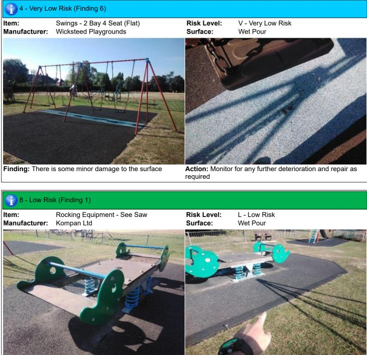
**Finding:** The surface is lifting at the edges and creating trip **Action:** Repair perimeter of surfacing to remove trip points
