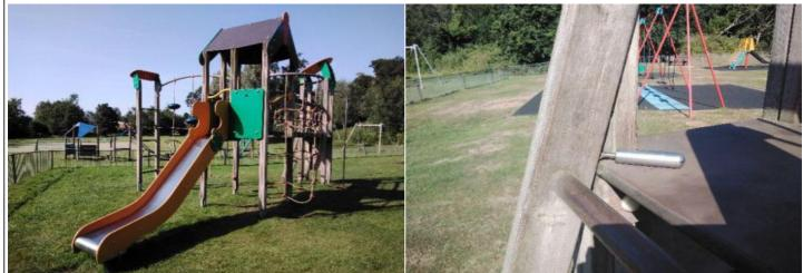
**Finding:** There is/are finger entrapment/s in the framework and the item fails to meet the requirements of BS EN 1176 Part 1 4.2.7.6 Entrapment of fingers
