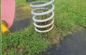
Finding: The U bolts clamping the spring are worn
