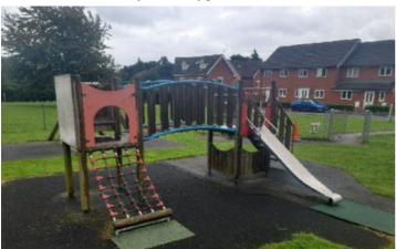
Finding: There is/are finger entrapment/s in the slide starting section due to missing inserts and the item fails to meet the requirements of BS EN 1176 Part 1 4.2.7.6 Entrapment of fingers
